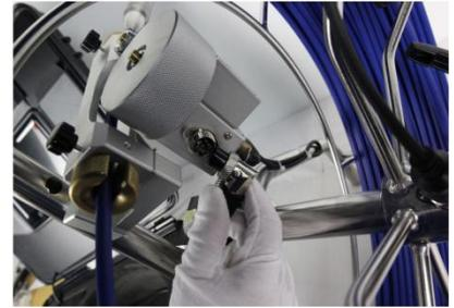
4. Release the coil brake
