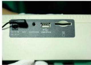
2. **Warning:** Pay attention to the direction of the SD card and plug it in reverse will damage the SD card
