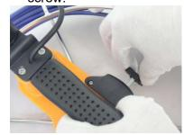
3. Clip the cable into the hook.
